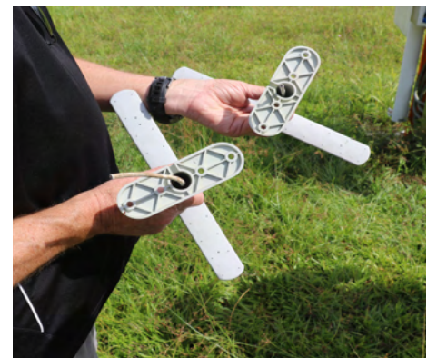
Above: The AWOS team fixes the vandalised weather station in Kokoda earlier this year Below: Damaged parts of the antenna at Kokoda weather station
